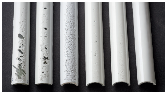
Comparison with different coatings after the erosion test.
